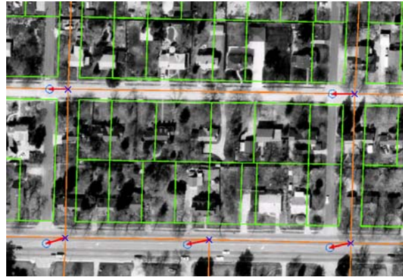
Figure 2. Finding the road intersection pairs: x symbol is location in vector database, and circle symbol is where it should be in imagery.
